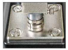
The standard base plate features four hole patterns for mounting fixtures; M4, M6, M10 and M12. An optional imperial base plate features #10-32, 5/16-18, 1/4-28, and 1/2-20. The base plate can be easily positioned to ensure correct sample alignment.
